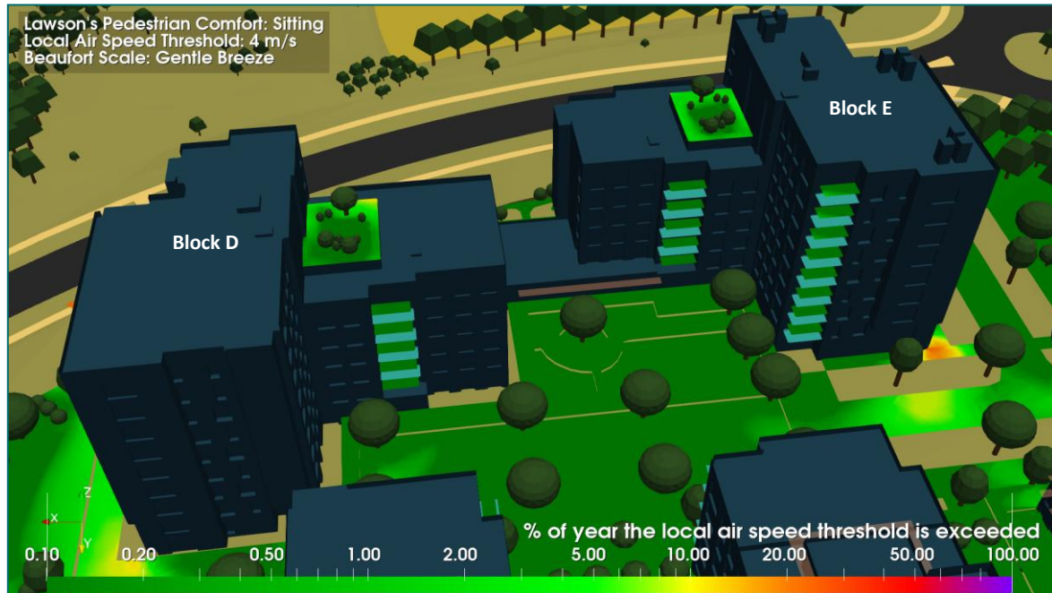
Figure 12: Sitting Comfort Criterion - Balconies - Block D & Block E (View from the North)
