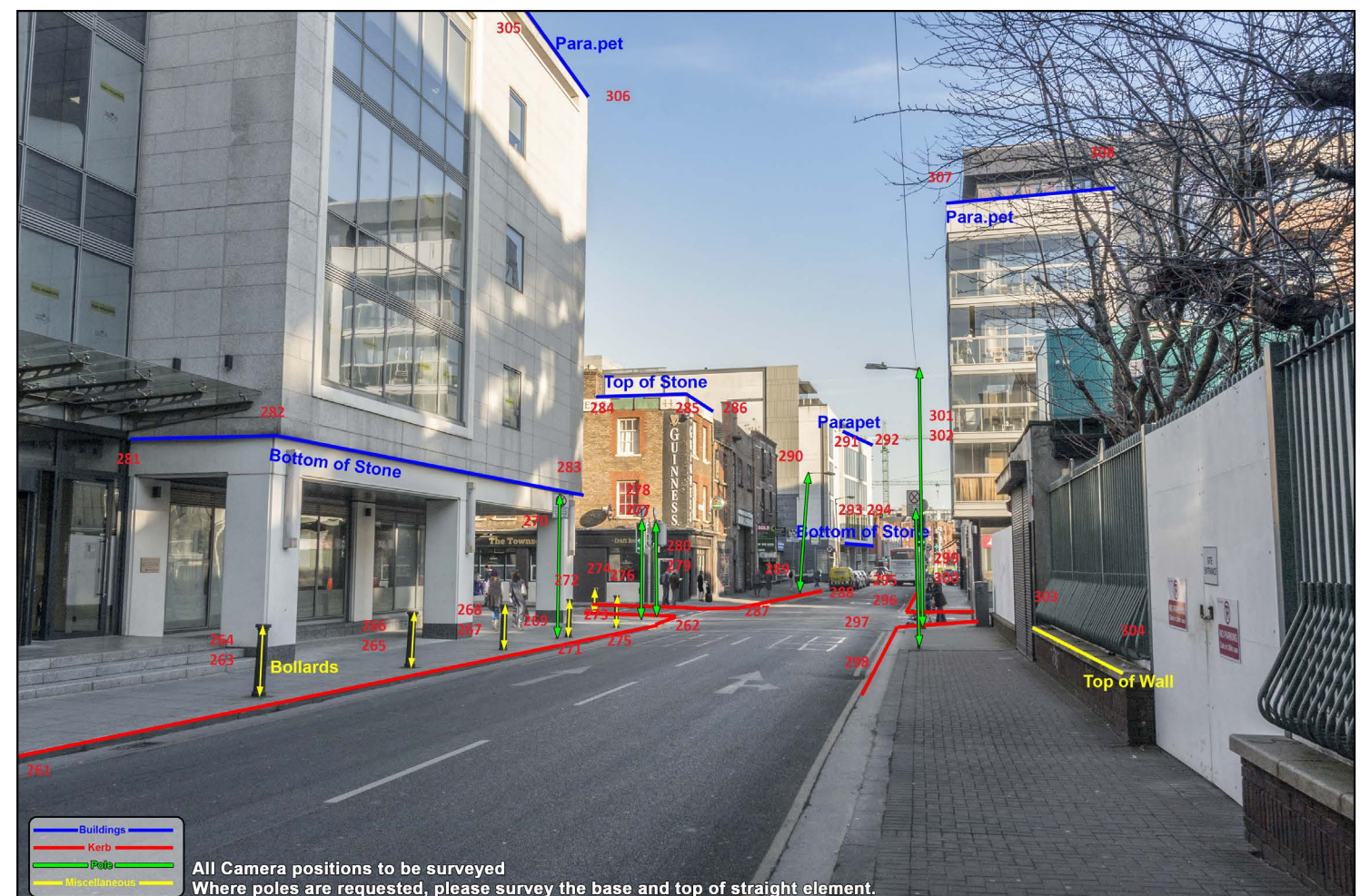
Fig.8: Fixed reference points fully surveyed and numbered.
