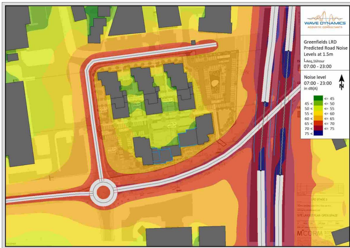
Figure 11: Predicted L_{Aeq,16hour} (07:00Hrs – 23:00Hrs) at 1.5m height for the future development.
