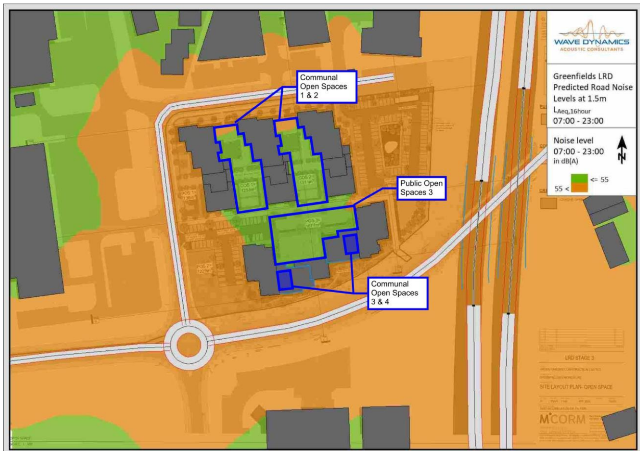
Figure 17: Indicative contour map displaying public/communal external amenity spaces within ProPG criterion.
